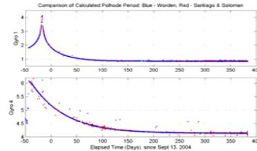
The polhode period of each gyro was observed to be changing over time. Each of the four exhibited similar asymptotic behavior. The only explanation that agrees with all the observation was that of energy dissipation in the rotor body. Dissipation moves the spin axis towards the maximum inertia axis where energy is minimum.
