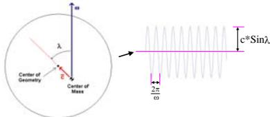
Mass unbalance creates a signal at spin frequency in the position as measured by the Gyro Suspension System (GSS). The amplitude of the signal is a function of both the length of the mass offset, and its angle to the spin axis.
