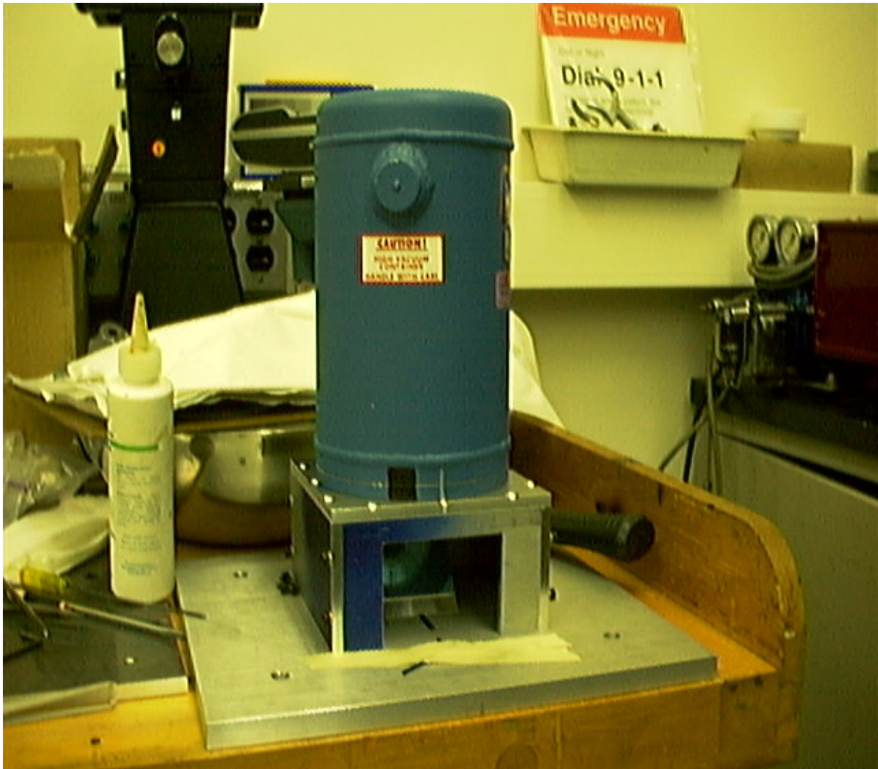
Dewar mounted on Shake Table Bracket with 45° deflecting mirror
