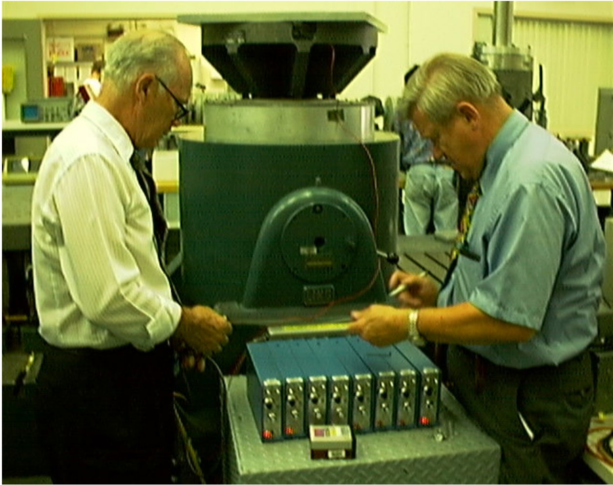
The Ling A300B Vibration Exciter & Shaker Table with Accelerometers and their amplifiers accompanied by qualified RQ&A personnel Howards Garrison and Menche in Bldg 244 at NASA Ames Research Center, Moffett Field, CA.
