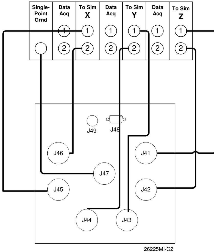
Figure 4. Connection of the FSU EU to Gyroscope Simulator Interface.
