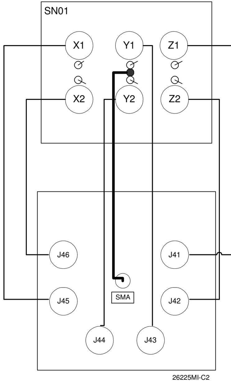
Figure 3. Connection of the FSU EU to Sn01 "Dummy Load".
