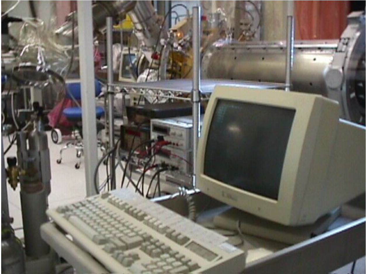
Photo 2 – Electronics set-up includes a Keithly electrometer for measuring the photo-current, a Keithly picoammeter for monitoring the lamp intensity and two HP DC power supplies which provide Hg lamp power as well as bias voltage.
