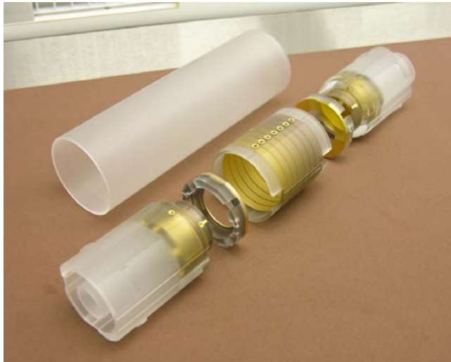
Quartz Housing Components and Test Masses \mu\text{m} Tolerances
