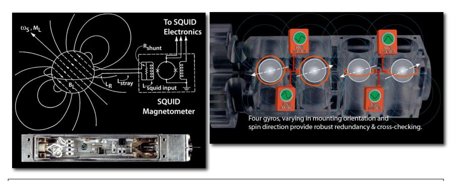
How can one monitor the spin-axis orientation of a near-perfect spherical gyroscope without any physical marker showing the location of the spin axis on the gyro rotor? The answer lies in superconductivity.
