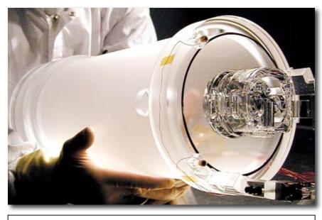
A telescope mounted along the central axis of the dewar and spacecraft provided the experiment's pointing reference to a "guide star." The telescope's image divider precisely split the star's beam into x-axis and y-axis components whose brightness could be compared.
