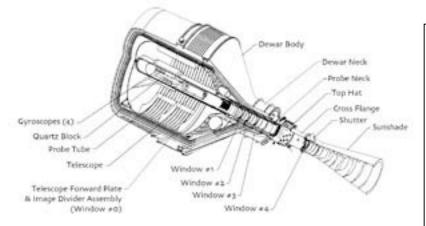
GP-B's 650-gallon dewar, kept the science instrument inside the probe at a cryogenic temperature (2.3K) for 17.3 months and also provided the thruster propellant for precision attitude and translation control.
