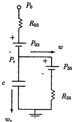
Fig. 8 Equivalent circuit of plenum pressure,  $P_c$ , dynamics.
