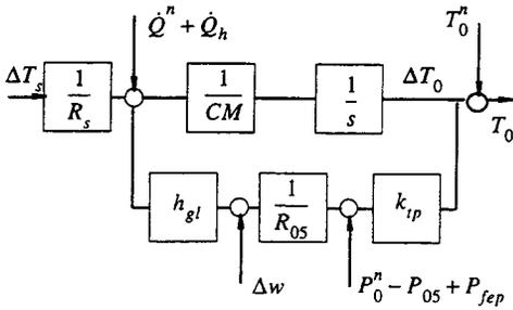
Fig. 4 Passive temperature control system block diagram.
