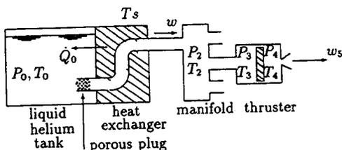
Fig. 2 Helium flow system schematic.
