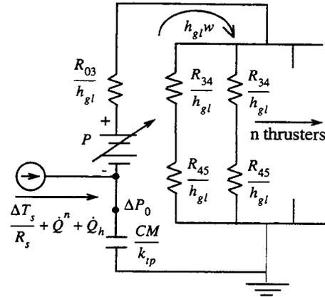
Fig. 5 Equivalent circuit depicting the thruster system thermodynamics.
