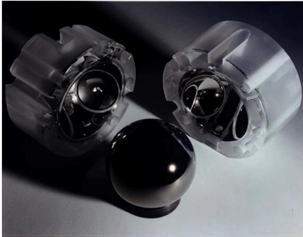
FIG. 2: A gyroscope aboard the Gravity Probe B satellite. Each gyroscope is a fused silica rotor about the size of a ping-pong ball, machined to be spherical and homogeneous to tolerances better than a part per million, and coated with a thin film of superconducting niobium. The gyroscope assembly sat in a dewar of 2440 liters of superfluid helium and was held at 1.8 degrees Kelvin. (Credit: Bob Kahn/Stanford University/Gravity Probe B)
