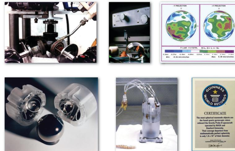
To measure the minuscule angles predicted by Einstein's theory, it was necessary to build near-perfect gyroscopes 10 million times more precise than the best navigational gyroscopes. The GP-B gyro rotors are listed in the Guinness Database of World Records as the most spherical man-made objects.
