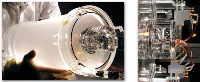
A telescope mounted along the central axis of the dewar and spacecraft provided the experiment's pointing reference to a "guide star." The telescope's image divider precisely split the star's beam into x-axis and y-axis components whose brightness could be compared.
