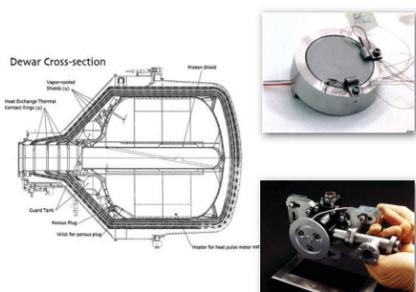
GP-B's 650-gallon dewar kept the science instrument inside the probe at a cryogenic temperature (2.3K) for 17.3 months and also provided the thruster propellant for precision attitude and translation control.
