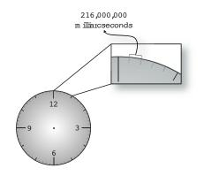
Gravity Probe B must be able to measure half of one of those milliarcseconds -- an angle nearly one five-hundred-millionth of the space between each minute mark!
