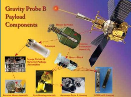
The slowly escaping helium also served as the propellant for 16 microthrusters that kept the spacecraft pointed towards the guide star, and maintained its drag-free position in orbit and constant roll rate. Outside the dewar, mounted to the spacecraft frame are all the systems that provide power, navigation, communication and control of the spacecraft.
