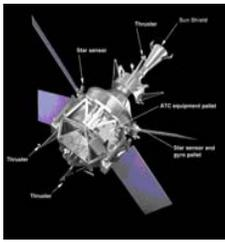
There are two star trackers onboard the GP-B satellite.
