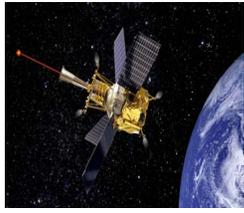
The GP-B satellite is controlled to roll with a period of 77.5 sec about an axis along the direction to the guide star.
