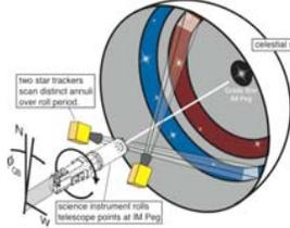
Ideal roll phase:  $\phi_{QB}(t) = \omega_{roll}t + \delta\phi_0$ , where  $\omega_{roll} = 2\pi / 77.5$  rad/sec and  $\delta\phi_0$  is constant.
