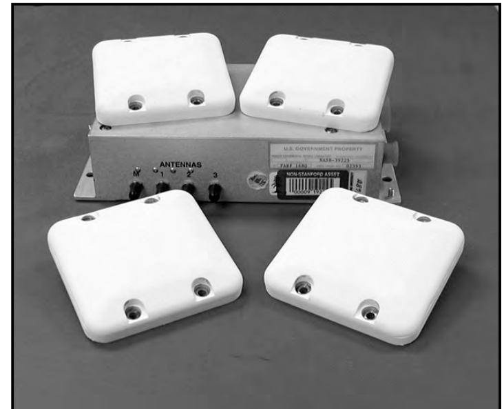
GPS Pathfinder unit with antenna array
