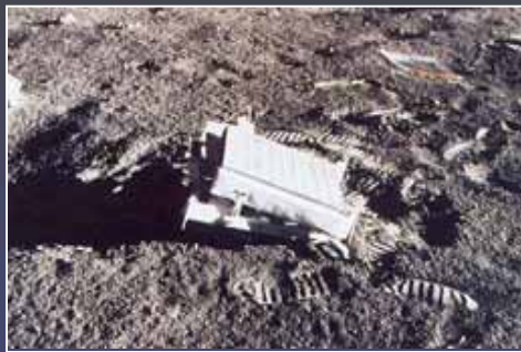
Laser Ranging: to reflectors on Moon (1968+)
