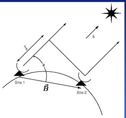
Combine measurements of fringe phase (and amplitude) from baselines (B) with different ("projected") lengths and orientations to produce a source brightness map
